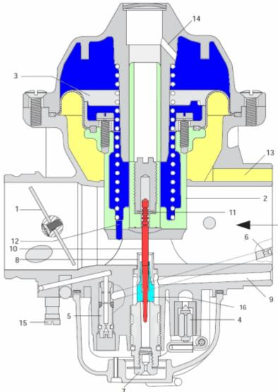
It is wrongly assumed that the diaphragm also ensures an adjustment of the mixture depending on the pressure in the Venturi tube (the narrowest point in the area of the nozzle block in the carburettor).
