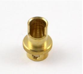
The 80 hp engine has a symmetrical atomizer (left). The upper end protrudes into the Venturi tube in a ring.
