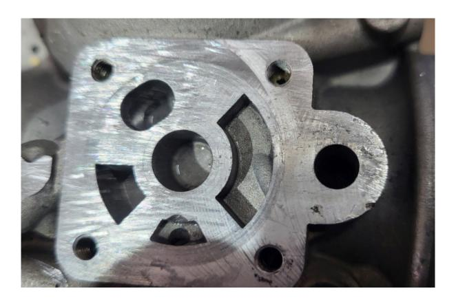
I suddenly remembered that I had stumbled across a carburetor housing like this before. I had seen exactly the same picture a few years ago in the course of a complaint. A milled edge on the carburetor housing reached into the area of the choke plunger where it is supposed to seal. As the rotary piston cannot fully rest and seal here, it is not possible to achieve good engine running with the leaking choke.
