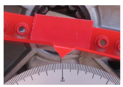
Turn the piston to the piston stopper at cylinder 2 and read the position on the degree disk.
