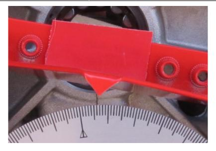
Here you can clearly see that the crankshaft is rotated by approx.  $6^{\circ}$  between the two measured cylinders, in this case between cylinders 1 and 2. The measured value for cylinders 3 and 4 was also  $6^{\circ}$ .
