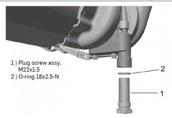
A strainer is integrated into the oil sump vessel here, which prevents carbon crumbs of one size from reaching the banjo bolt of the return line, which can clog it.
