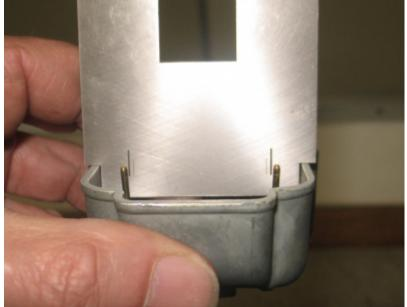
**In the left picture** you can see the millimeter division for the float level. Here you can also see the difference between the two arms of the float suspension on the other side.
