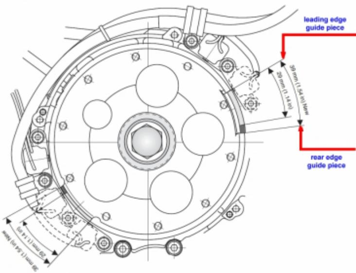
When the engine is started at a starting speed of approx. 350 rpm by the starter motor, this pulse is triggered at the trailing edge of the guide pieces. This was 4° before TDC on the older version of the solenoid hub and is 3° after TDC on the solenoid hub for the soft start modules.
