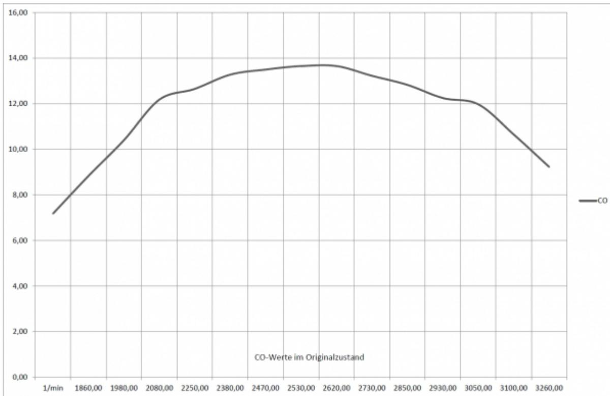
**The CO values** should not exceed 14% if possible, otherwise the engine can no longer “process” the mixture that is too rich for it and starts to shake. However, this is not caused by increased
