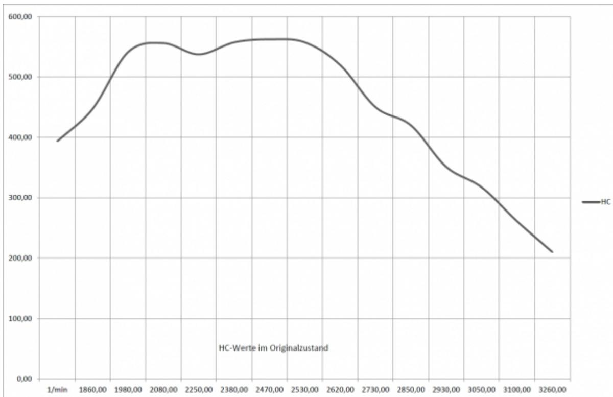
**The HC values** indicate unburned hydrocarbons - which may also contain oil. The diagnosis of increased oil consumption in connection with the CO values is to be seen here. In principle,
