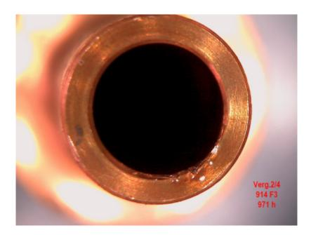
A flared edge can be clearly seen on the needle jets **with 206 operating hours**, which is caused by the constant beating of the jet needle when the carburetor vibrates.
