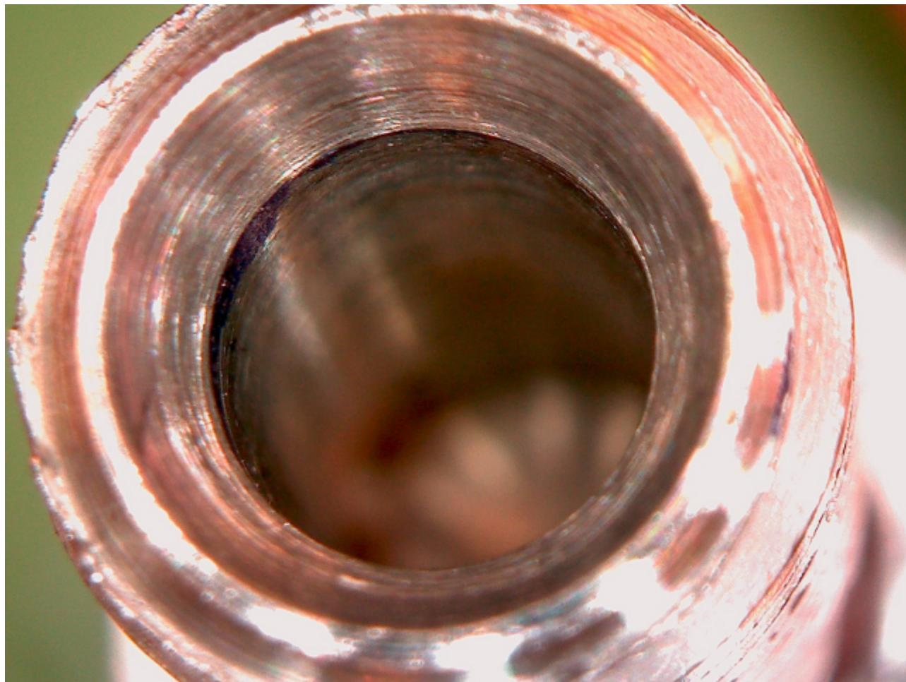
The image shows the conical valve seat in the banjo bolt. You can imagine that a leak is pre-programmed here.
