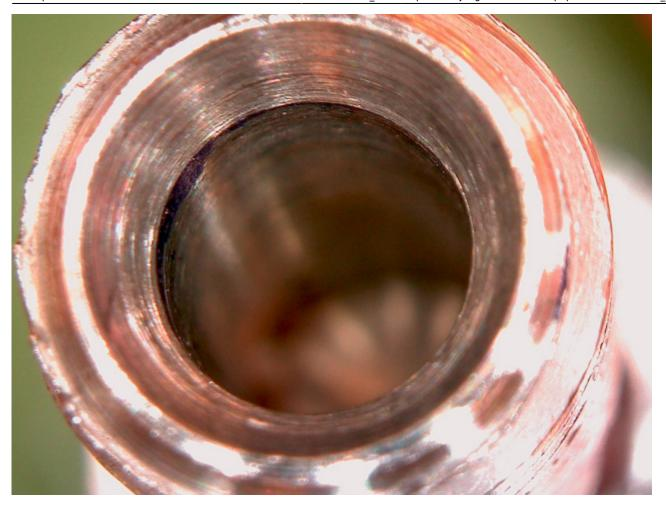
The image shows the conical valve seat in the banjo bolt. You can imagine that a leak is preprogrammed here.
