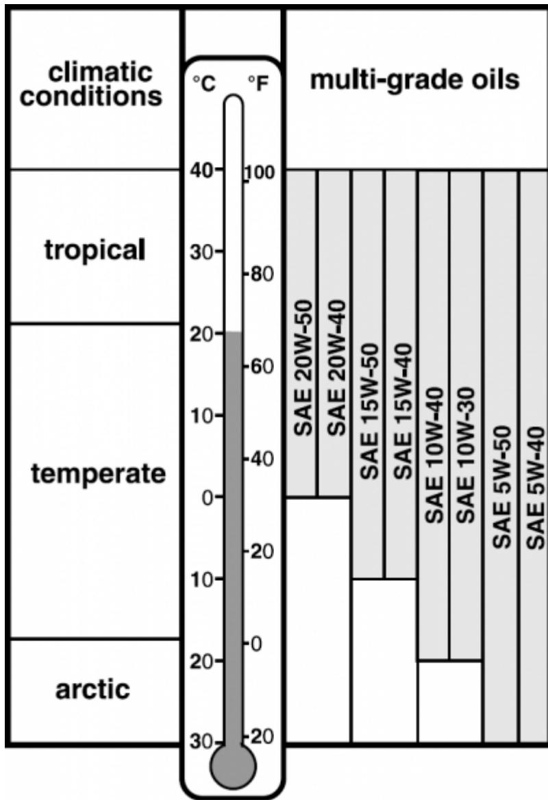
First of all, there is the selection of the engine oil and the viscosity (see image). If the starter is to crank the engine even in extremely cold conditions, an engine oil that is as thin as possible at this temperature is more than helpful. On the other hand, the oil naturally becomes quite thin at high oil temperatures and may lead to reduced oil pressure. But that's another topic.
