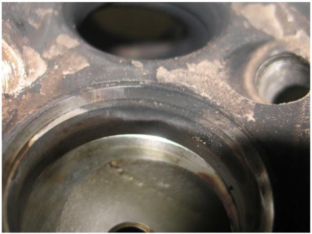
Here we can clearly see a black area on the inlet valve seat. The valve is no longer working properly there and the combustion gases are escaping. Here we have the measured pressure loss.
