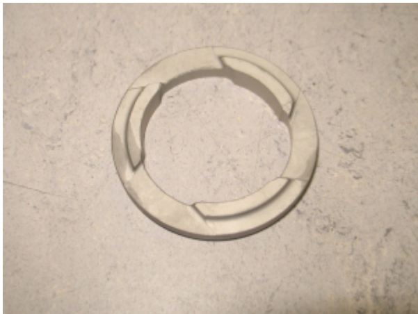
1st picture: Prototype of the stepped sleeve - 2nd and 3rd picture: The final shape.
