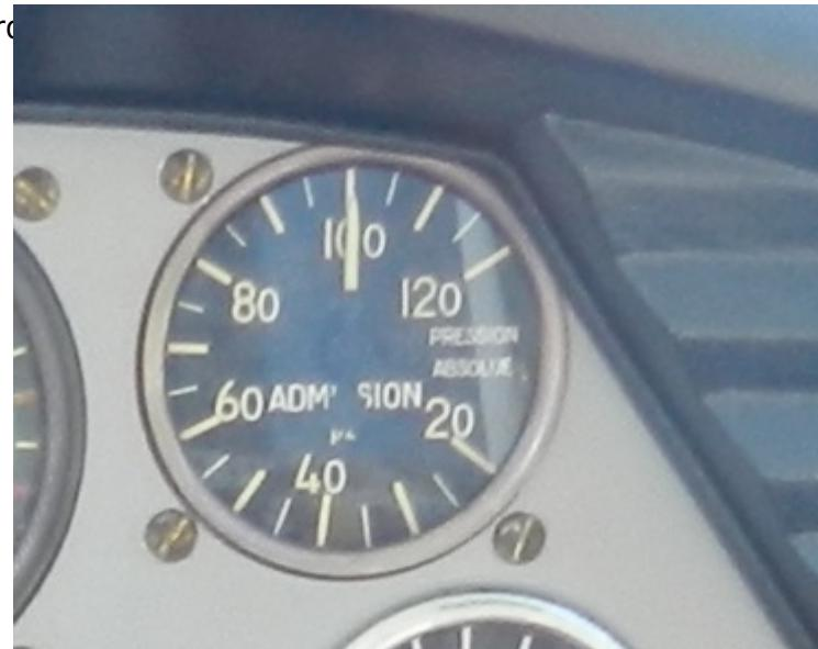
Unfortunately, the instrument cannot be used for a Rotax and it seems to me that this is a boost pressure gauge with a scale tailored to the engine. As you can see, it shows 100% when the engine is stationary, which corresponds to the ambient pressure.
